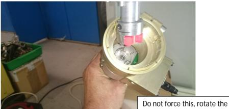
encoder whilst fitting to ensure alignment
